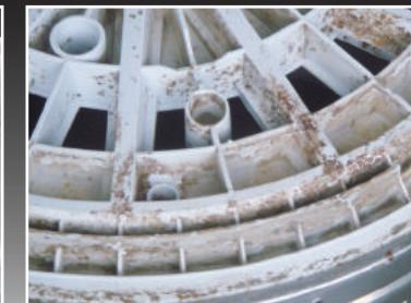
Dirt on the outside of the stainless steel tub
