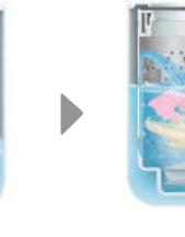
The third level of water assures that the detergent comes into complete contact with the surface of clothes.
