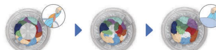
When the spin cycle ends, clothes remain pressed against the drum and are difficult to take out
